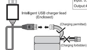
7.4V 2000mAh Li-ion (Enclosed)
