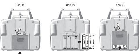
ATTENTION: Batteries shall be put to the right polarity.
